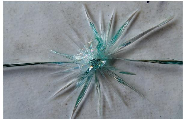
**Figure 17** A star or X-shaped fracture. This sample was from the lower of two layers of glass. The top layer displays a faint “lotus” flower from the impact.
