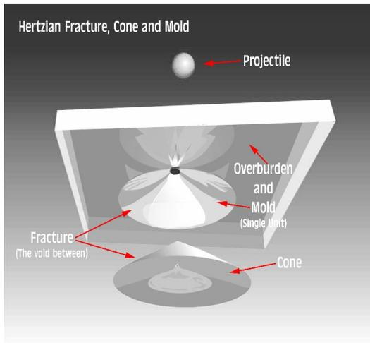
**Figure 3** Diagram of the three main segments of a simple Hertzian fracture in a glass plate; overburden and mold, fracture and cone.
