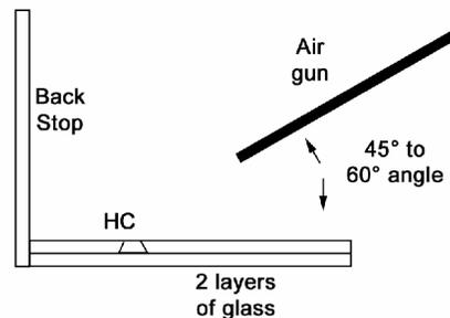
**Figure 2** Configuration of impact sample set.
